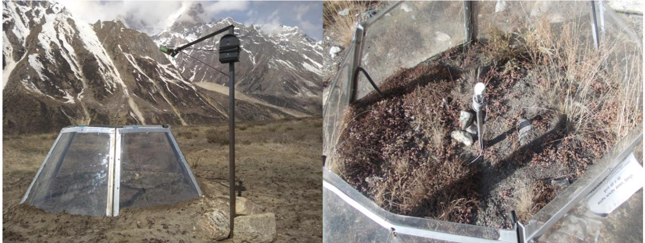
Fig. 4 Installation of Open Top Chamber
